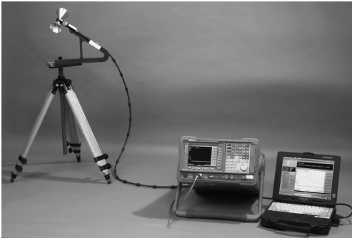
Figure I.4.3.: Typical spectrum analyzer measurement kit
